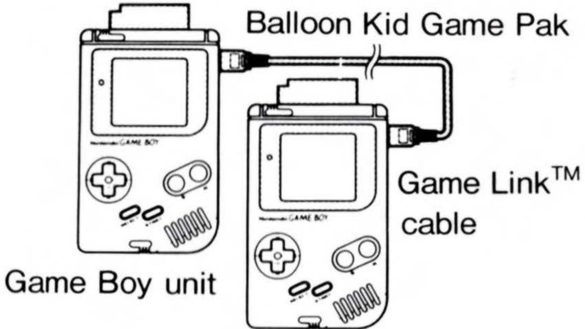
Connect the Game Link<sup>™</sup> cable as shown in the diagram. After checking that both Game Paks are set properly, turn on the power switch on both units.
